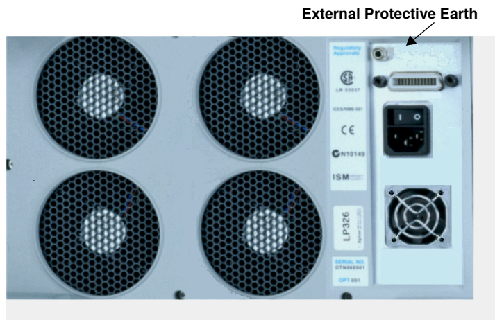
Figure 1 Earthing terminal - rear panel
